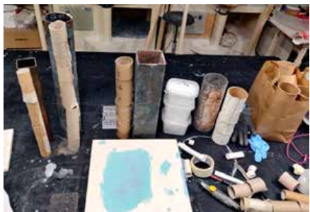
Figure 3 The layering process consists of three parts: firstly, positioning discarded cardboard rolls that serve as a frame for the glass powder; secondly, alternately applying glass powder and sand to create a stalagmitic shape; and thirdly, positioning the outer metal mold, which holds the mixture of sand and glass in place and prevents it from shifting during firing (Photo credits: Meta Mramor).
