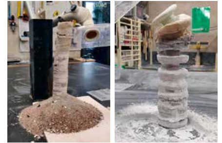
Figures 4 & 5 After firing in a glass kiln, the glass powder turns into a solid structure that can stand on its own. The outer metal mold and sand are removed and reused to produce the next object (Photo credits: Meta Mramor).
